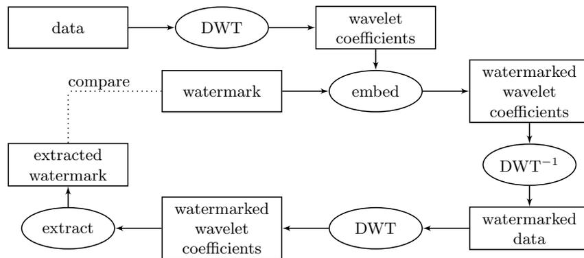
Fig. 1: Generic scheme of watermark embedding and extraction in the wavelet transform domain.
