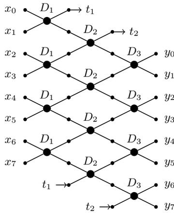
Fig. 2: Lattice structure performing 6-tap transform.
